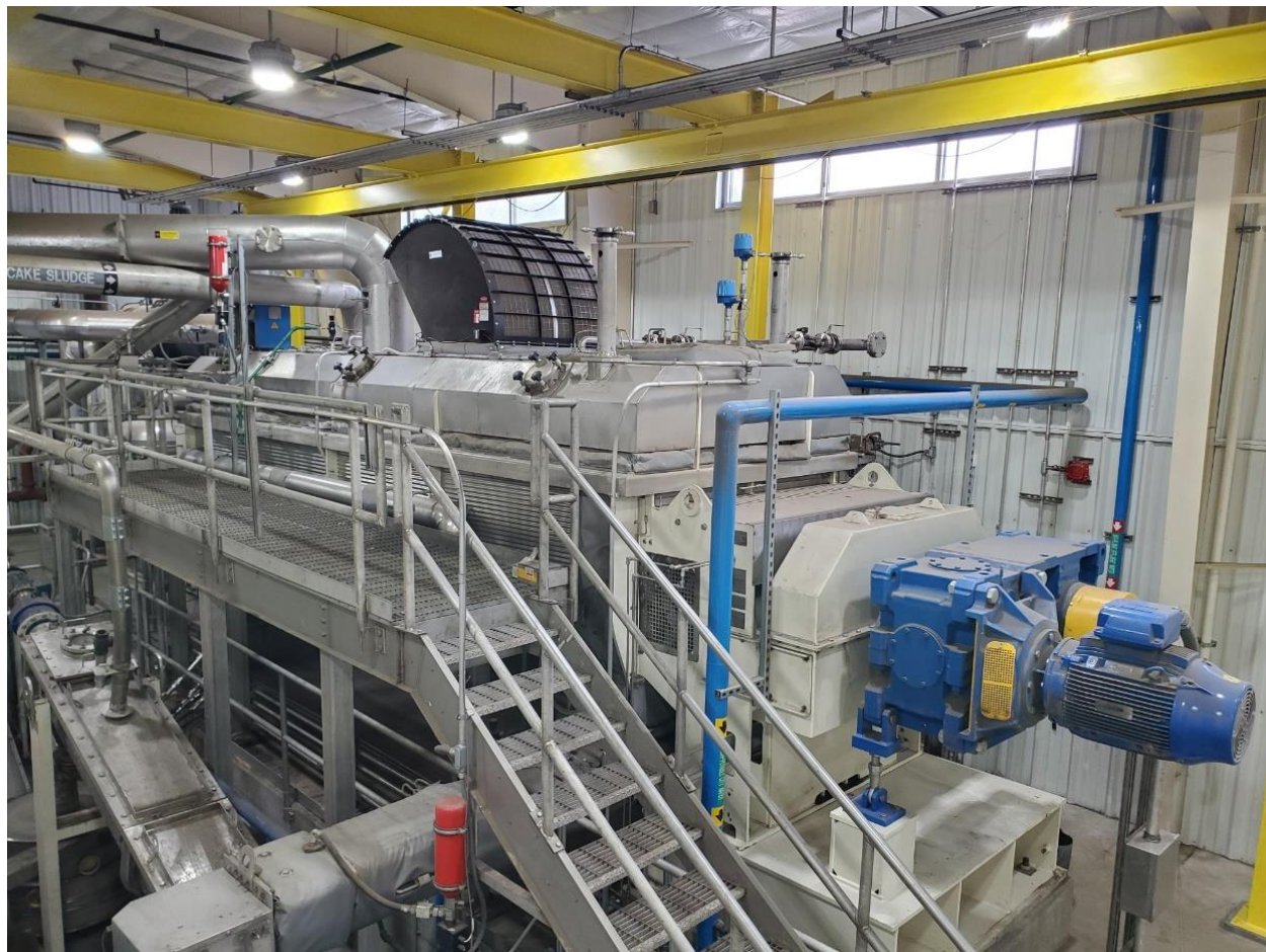
Figure 2. Andritz 10W-310 Biosolids Paddle Dryer. Source: City of Stevens Point.
